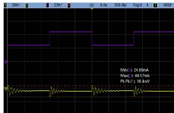
**Figure 9: Small-Signal Load Step and Voltage Response**
