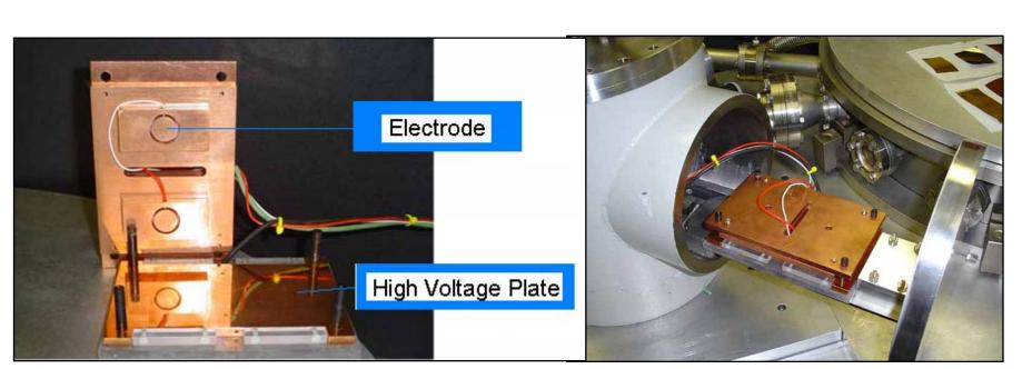
Our Constant Voltage Apparatus is capable of measuring currents in the femto-amp range. This allows materials with unusually high resistivities to be measured. Samples are carefully cleaned, mounted, and vacuum-baked before placement in the chamber. (Base pressure < 10<sup>-4</sup> Torr.
