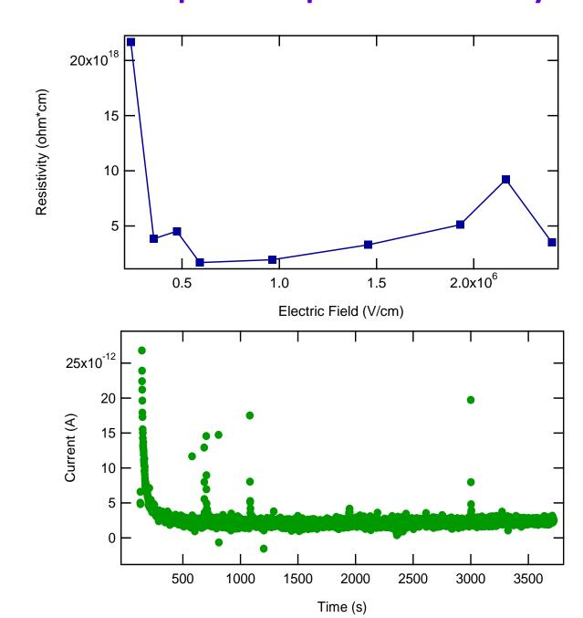
The top graph is an example of a data set for determining the resistivity. The current approaches an asymptotic limit, and it is this current which is used to calculate the material's resistivity. The resistivity is somewhat dependent on electric field magnitude (shown in graph above to the right), but the effect is relatively small, typically less than an order of magnitude. The average resistivity of Kapton E has been determined at 3 x 10<sup>18</sup> ohm·cm.
