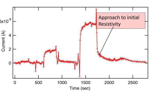
Resistivity of an irradiated Kapton E sample was tested 16 days after radiation exposure, to look for long term effects. No electric field had been applied to this sample during irradiation. Using the constant voltage method, we determined the resistivity at several electric field strengths (table at right). The average measured resistivity was a full order of magnitude less than that exhibited by unexposed Kapton E.
