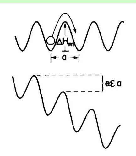
The theory of thermal assisted hopping conductivity, developed by Mott and Davis, provides a model for the temperature and electric field dependence of the dark current conductivity of materials.
