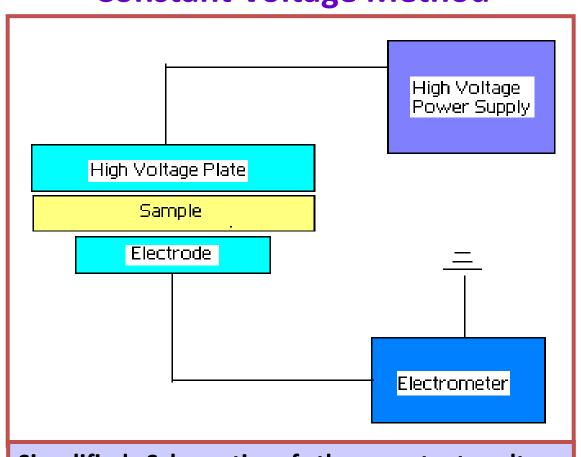
Simplified Schematic of the constant voltage method. A thin polymeric sample, sandwiched between two plates is subject to an electric potential, driving current through the sample. A high resolution electrometer measures the current, and thus resistivity may be calculated.
