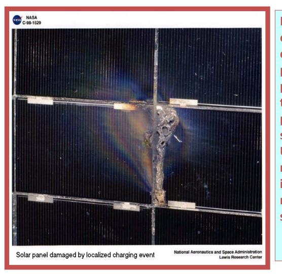
Interaction with the plasma environment induces spacecraft charging. Electron, ion, and photon charge-induced potentials can result in arcing, thus damaging electronics, solar panels (at left), or other spacecraft components. Understanding how charge migration and dissipation occurs in insulators is crucial to mitigating the effects of spacecraft charging.
