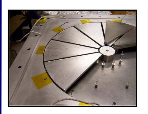
The apparatus used to make RIC measurements included the vacuum chamber, interior of which is shown to the left. Using a combination of a picoammeter and a multiplexer, data could be taken simultaneously on 10 different large area, thin polymer samples.
