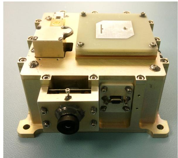
**Figure 2: Camera assembly and SSBV CubeSat ADCS experiment on TechDemoSat-1.**
