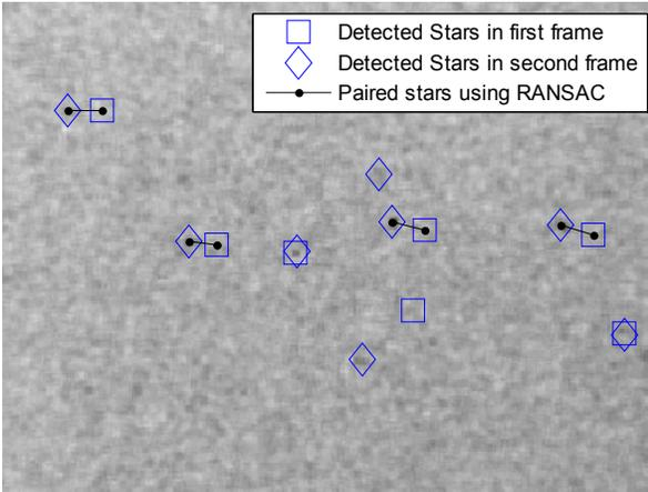
**Figure 5: Processing and star pairing of two overlaid images 1.5° apart. Image is cropped and colors are adjusted for clarity.**
