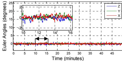
**Figure 7: Euler angles representation of attitude difference between estimated and actual attitudes for a MEMS gyroscope rate integrator assisted by a stellar gyroscope. The stellar gyroscope resets the drift every 15 seconds, at least two stars common to the field of view throughout the plot duration are assumed.**
