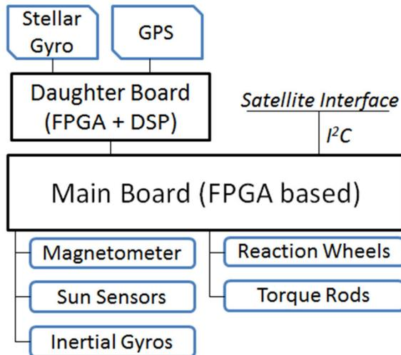
**Figure 1: Top: photos of the CubeSat ADCS board of both faces with daughterboard installed (prototype hardware with test connectors). Bottom: block diagram of the overall system.**
