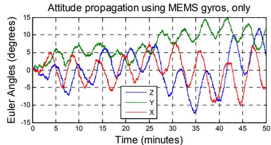
**Figure 6: Euler angles representation of attitude difference between estimated and actual attitudes for an unassisted MEMS gyroscope rate integrator. Beginning with perfect knowledge, the plot illustrates attitude loss in eclipse.**
