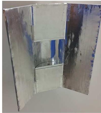
**Figure 18: Physical Model of 3U Parabolic Antenna with Deployable Extended Reflector**
