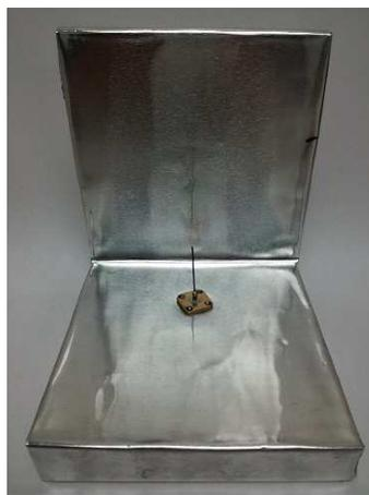
**Figure 4: Physical Model of 1U Reflector Antenna with Radiating Monopole**
