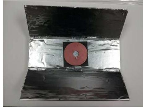
**Figure 25: Physical Model of Annular Ring Patch Antenna**
