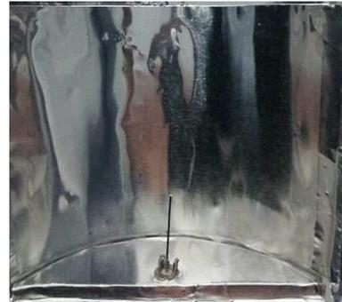
**Figure 14: Physical Model for Monopole with Parabolic Reflector**
