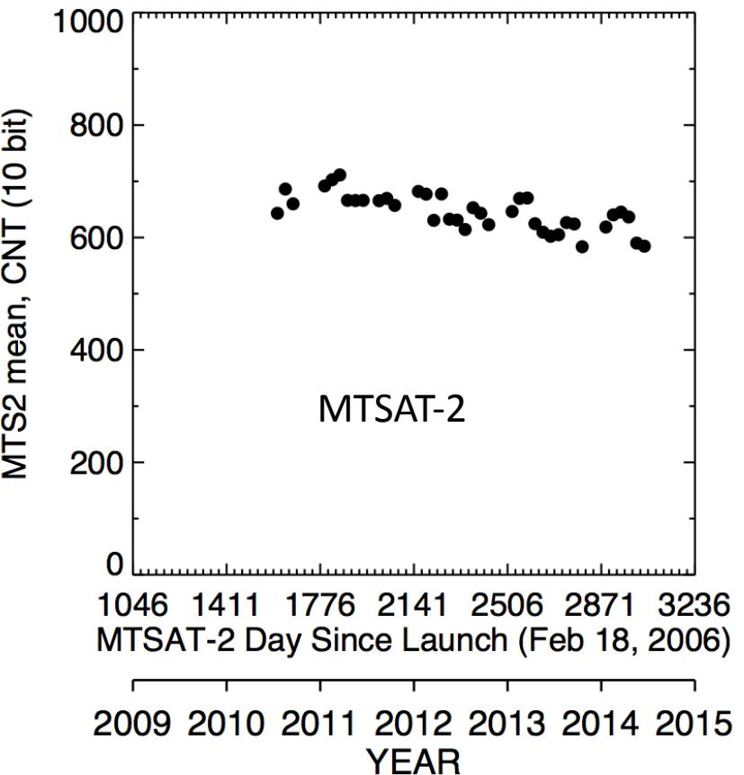
Easily monitor the degradation of the MTSAT-2 monthly mean DCC counts
