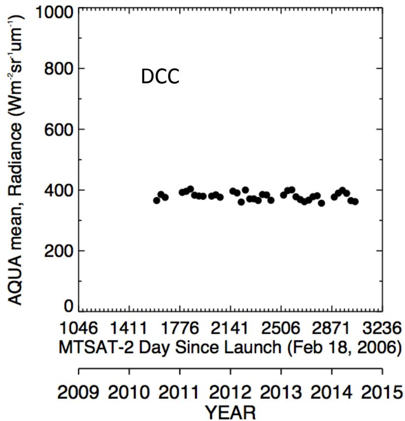
The stability of the monthly mean MODIS radiances reveal that DCC are stable targets if analyzed collectively (Must have maintained sun-synch orbit)
