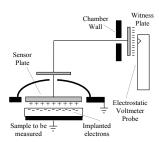
Figure 2. Detail of the capacitive measurement system used
