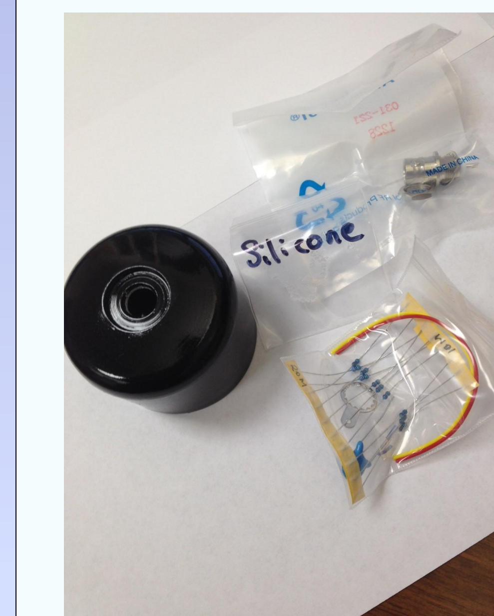
Fig. 6 BNC Mounting apparatus for PMT
