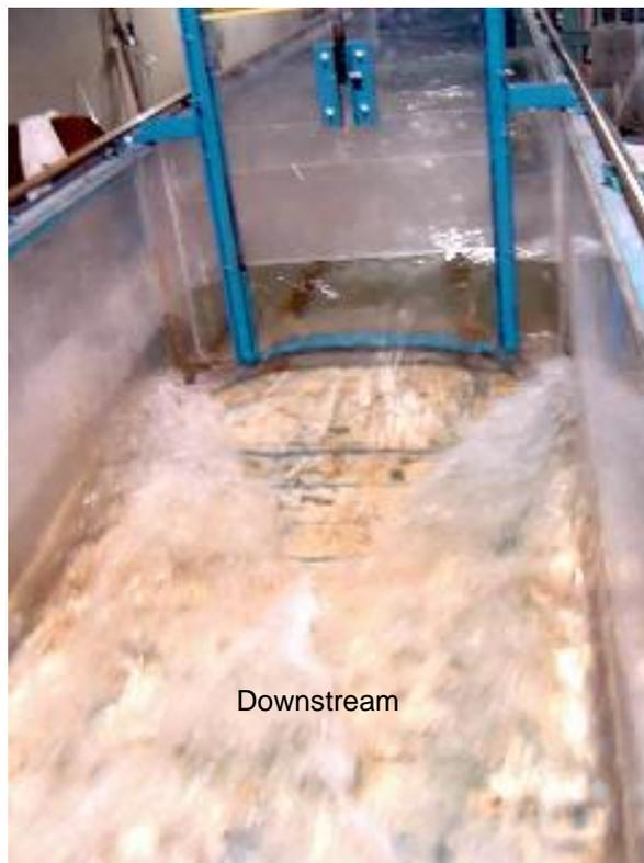
**Fig. 10.** Laboratory photograph showing an example of a free non-orifice flow regime
