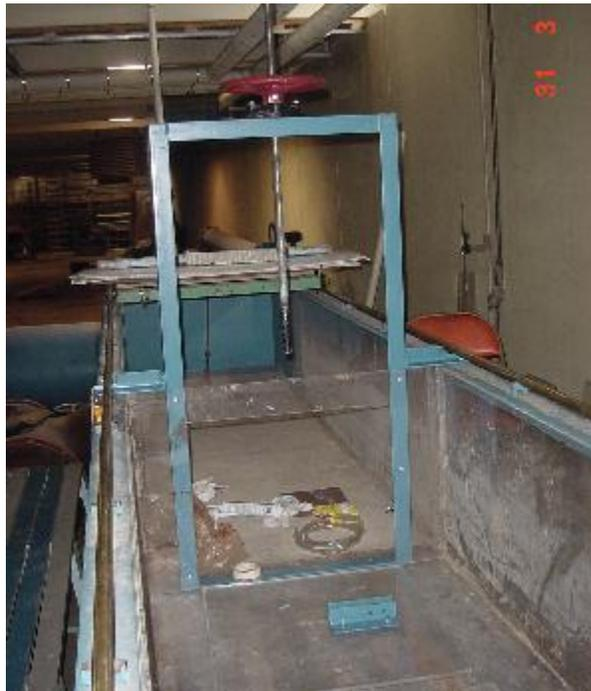
**Fig.40.** Gate after installation in the rectangular flume
