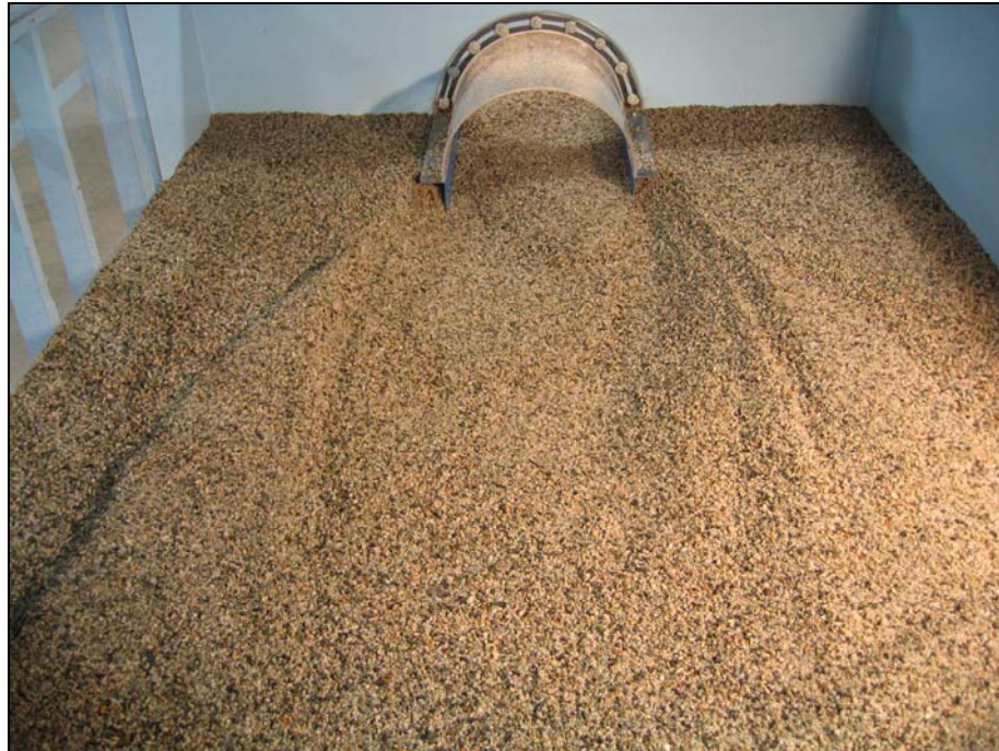
Figure 42. Example of scoured channel at culvert exit with bank deposition.
