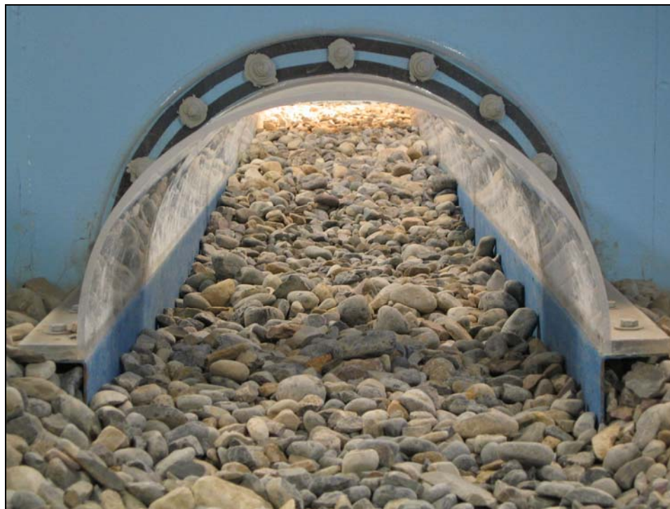
Figure 53. Scour of 2-inch cobbles looking upstream from exit.
