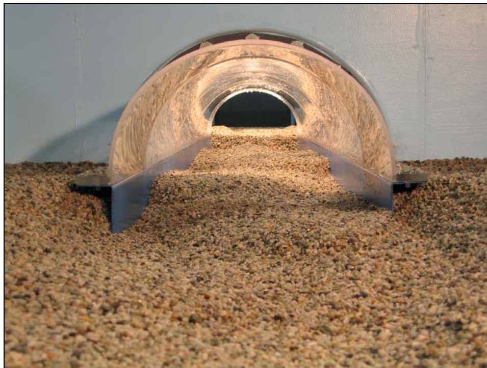
Figure 44. Example of antidunes in pea gravel substrate.
