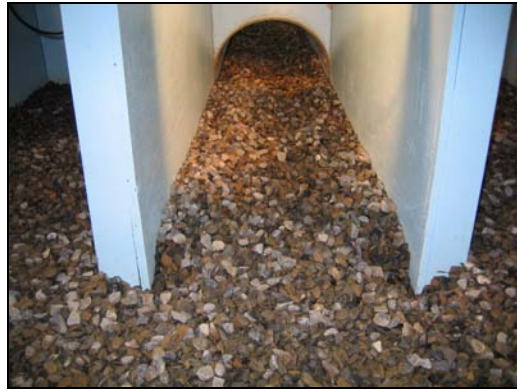
Figure 8. 0% Contraction with headwall.
