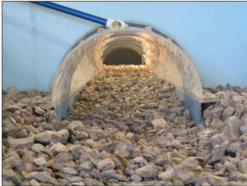
Figure 58. Scour of 2-inch angular rock looking upstream from exit.
