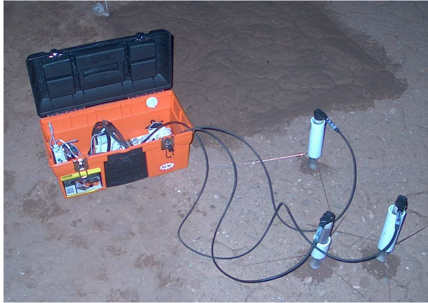
Fig. 5.1. Three minidisk infiltrimeters connected to a HOBO U12 data logger.
