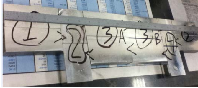
Figure 10. AA-6061 mirror blank center slice cut up into twelve smaller pieces for hardness measurements
