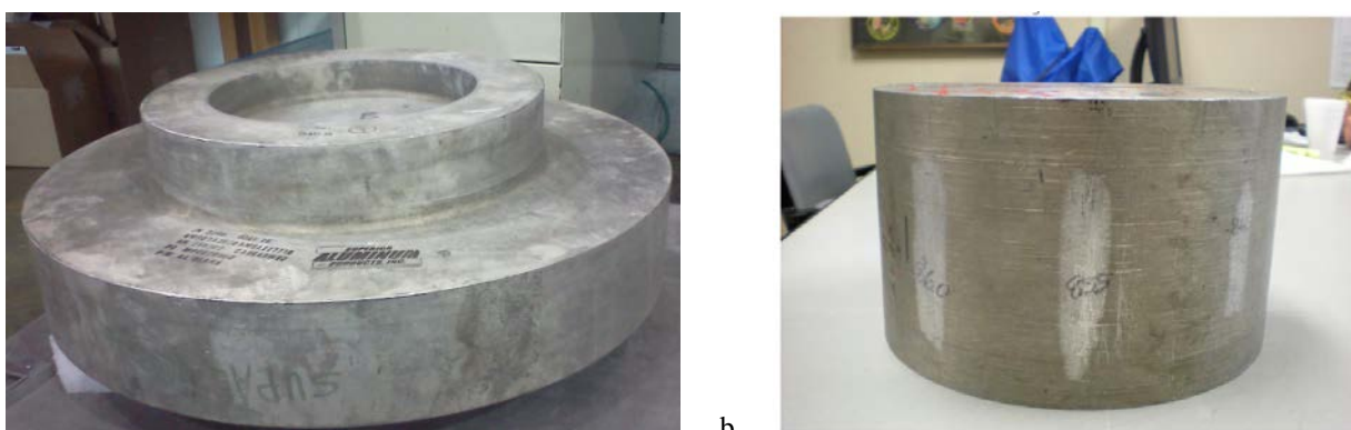
Figure 4. a) Conventional AA-6061 test blank. b) Melt spun RSA-6061 test blank.
