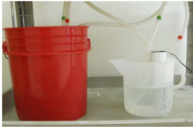
Figure 5: Final prototype. Note the addition of a PVC chamber for the sensor, this was added to prevent hose and foam interference with the sensor.
