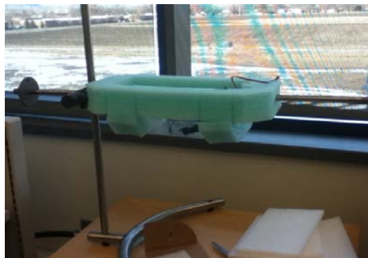
Figure 3: An over bucket mounting scheme. This design was ruled out due to needless complexity, instability, and potential for contamination.
