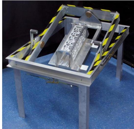
**Figure 2: Pitch-Roll Apparatus to Perform Ground-Based Calibration of CubeSat**
