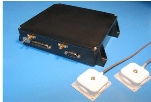
**Figure IX: A replacement for the SGR-10 Space GPS Receiver will make use of SGR-ReSI core**
