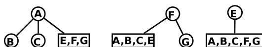
Figure 3.6. Without any knowledge of node D , this is as far as the algorithm can get. Because the forwarding tables of all three trees contain all the nodes from the other two trees, it is obvious that they are connected via an unknown bridge.
