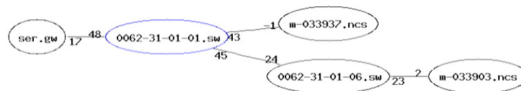
Figure 6.5. A localized map of the network. This example happens to contain a router, two switches, and two wireless access points.
