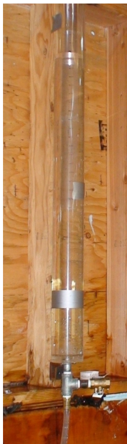
Figure 7. Reservoir piezometer with measurement scale.
