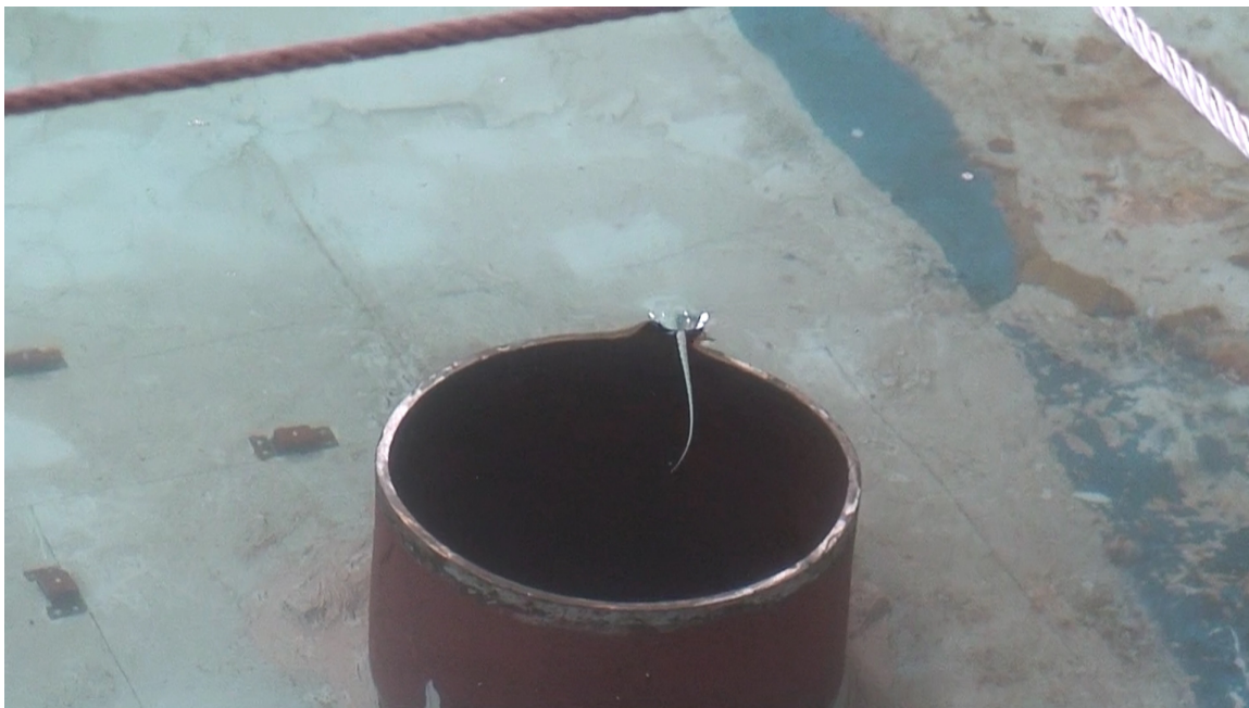
Figure 15. Open configuration with air-core vortex.
