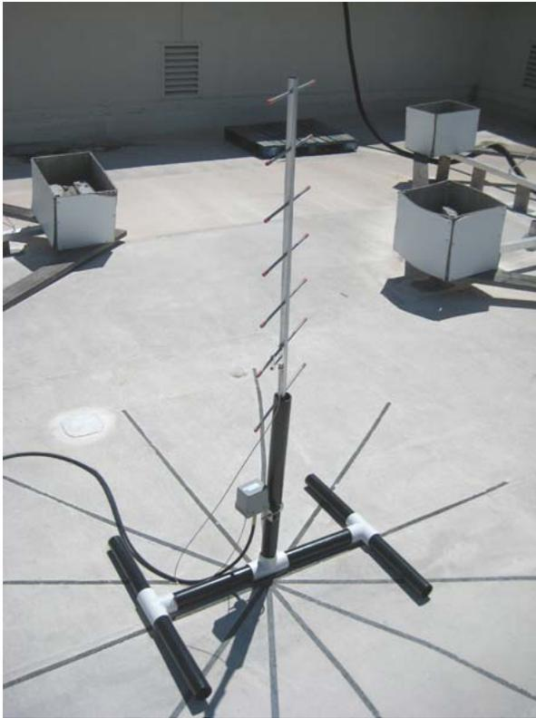
**Figure 15: A Beacon Station Antenna, using a vertically aligned 7-element Yagi antenna.**
