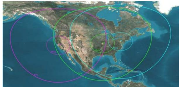
**Figure 14: Beacon Receive Station Locations, showing the 0 degree and 40 degree elevation masks.**
