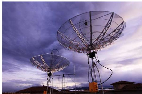
**Figure 5: Two S-Band Communication Stations installed at SCU, using 3-meter parabolic dishes. A dual-Yagi amateur radio station, used for high-gain beacon reception operations is seen in the background.**
