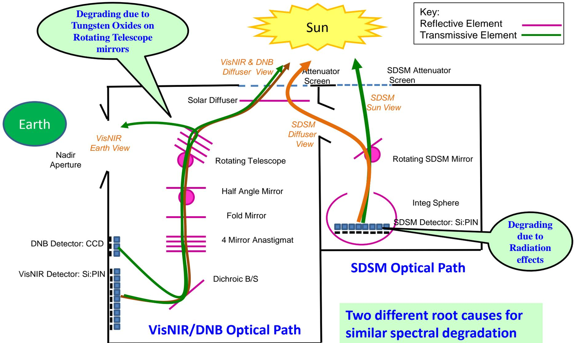
**Two different root causes for similar spectral degradation observed on-orbit**
