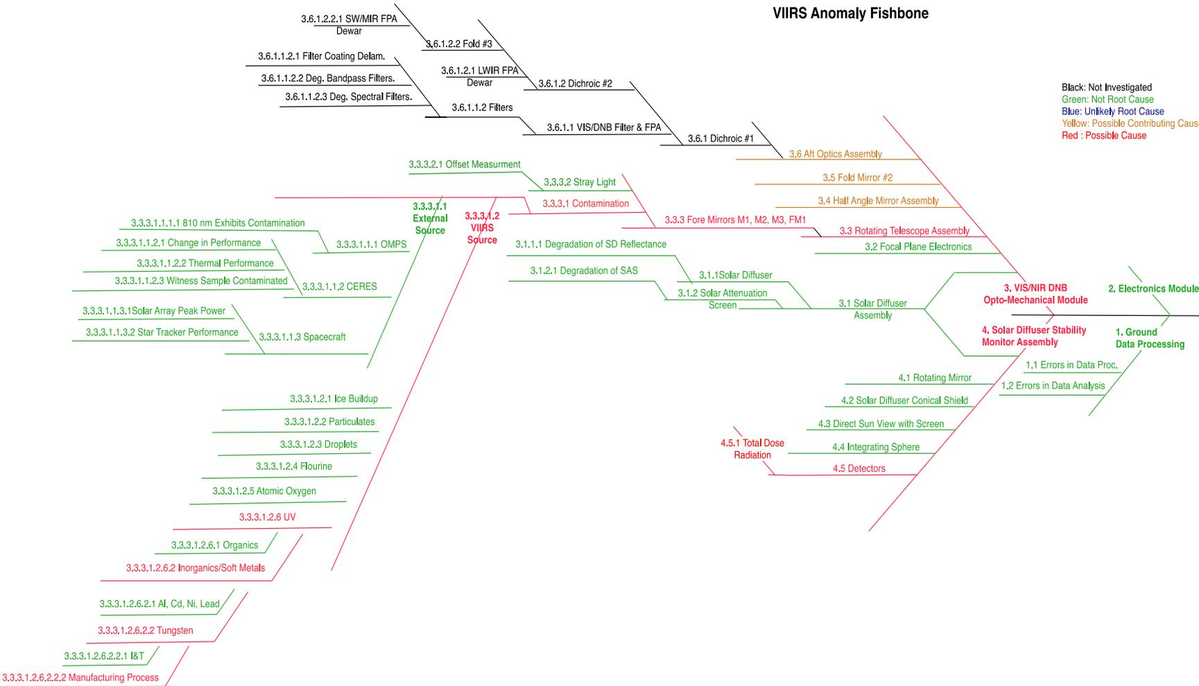
**VIIRS IR Band Degradation**
