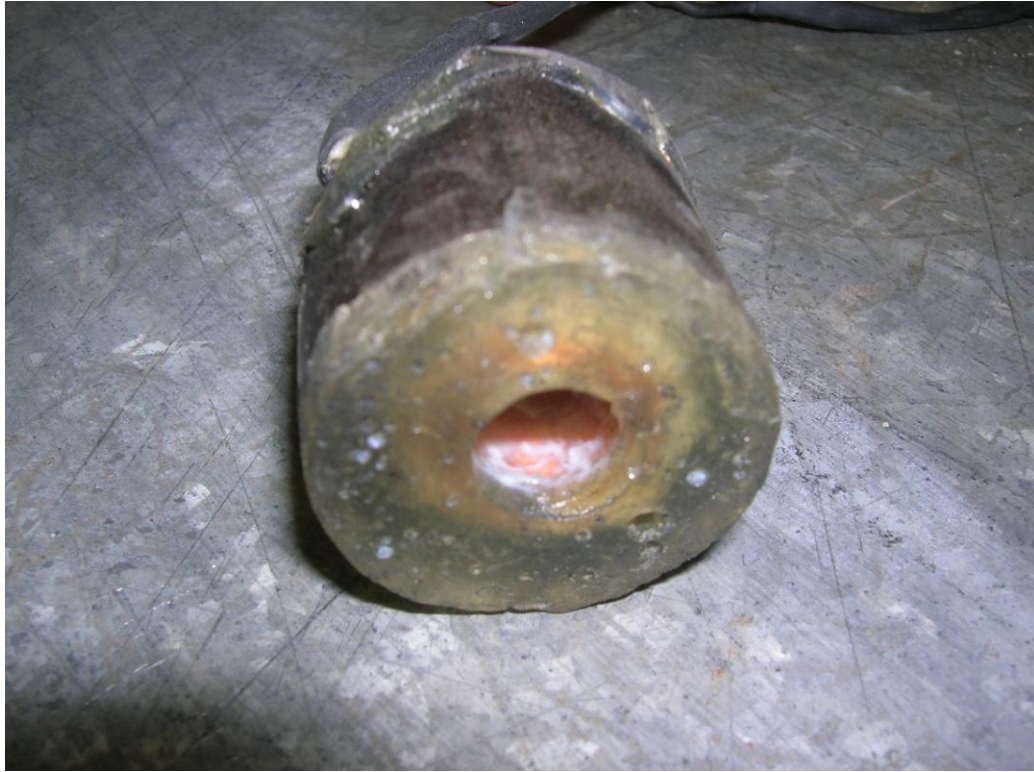
Fig. 5.6. Steel housing with epoxy protection
