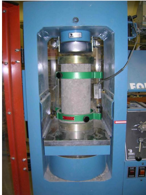
Fig. 7.4. Concrete cylinder instrumented with a compressometer and LVDT
