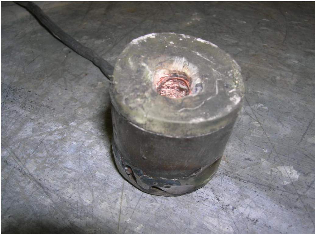
Fig. 5.7. Coil crushed inwards
