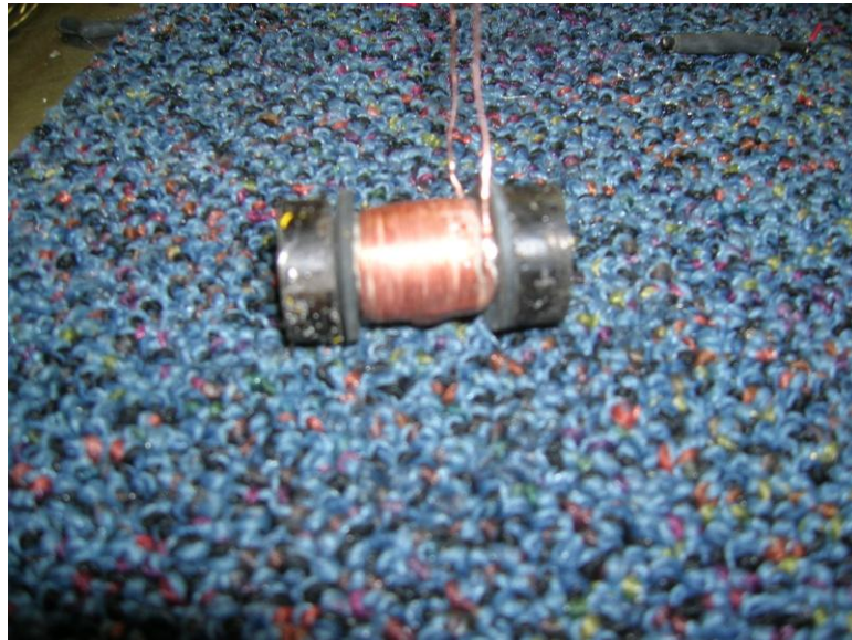
Fig. 5.4. Copper coil with steel end plates
