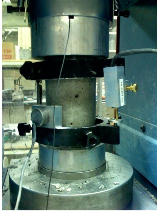
Fig. 5.10. Final configuration for experiment (LVDT on right, excitation device on left)
