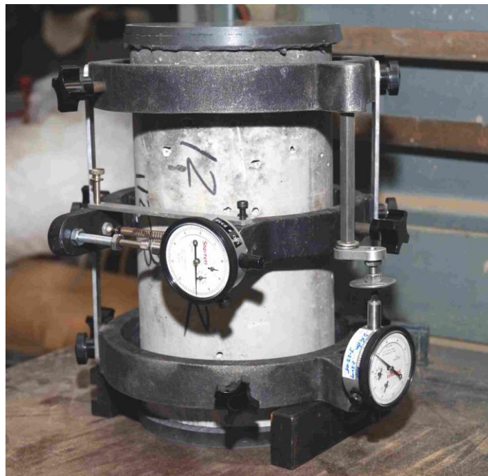
Fig. 7.2. Concrete cylinder instrumented with an extensometer and compressometer
