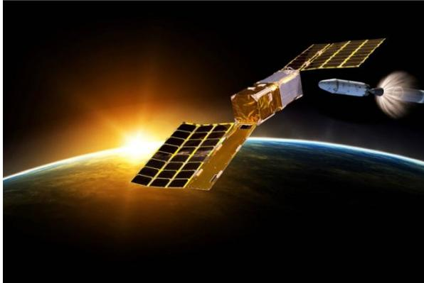
The system was designed to test a set of nanosatellite components in space. Following standard specifications, nanosatellites easily combine with one another onto existing rockets, and only require low development costs, making space mission participation more accessible to those outside the industry.
