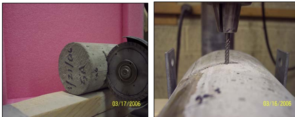
Figure 3.3. Procedure for making cuts on cylinders.
