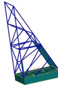
**Figure 7: Illustration of payload compartment and sunshield structure**
