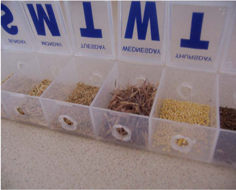
Figure 3.1. Ant specific seed tray fashioned from 7-day pill box. 10-mm entry holes were drilled into both outside walls of each compartment 5 mm from the base to allow free access by ants to seeds yet prevent the spilling of seeds out of the compartment and denying access to rodents.
