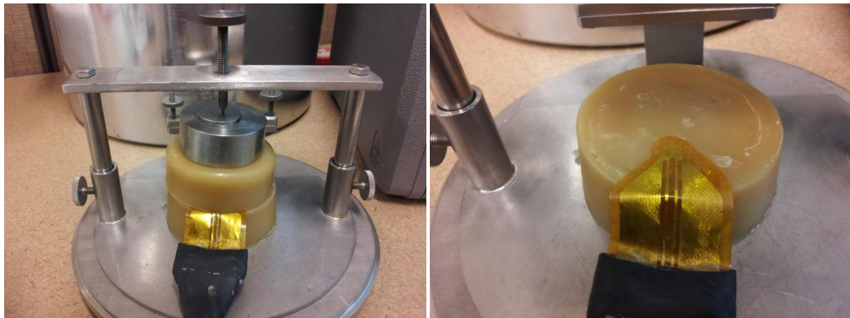
Figure 4: HotDisk© Experimental Set-up for Measuring Solid Thermal Properties
