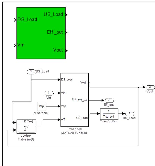
Figure 5: DC-DC Converter Model for use in the SimuLink® Analysis
