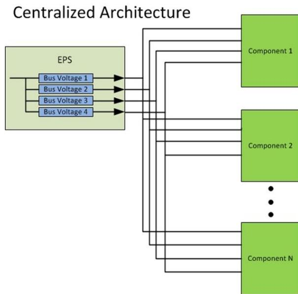
**Figure 1: Electrical Power System Centralized Architecture**
