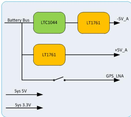
Figure 3: DICE ADCS Power Block Diagram
