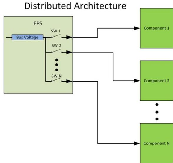
**Figure 2: Electrical Power System Distributed Architecture**
