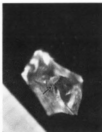
Fig. 29. Groove (arrow) produced by wire in reinforced window glass.
