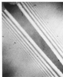
Fig. 36. (left). Interference pattern from moulded container. Note irregularity of pattern of approximately parallel fringes.
