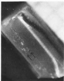
Fig. 30. Scratches (arrows) on rim of 'Pyrex' basin.
