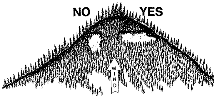
Figure 41 —Clearcut unit boundaries laid out across the slope that expose the short dimension of the unit to the wind help reduce blowdown.
