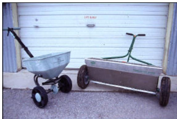
**Figure 3.** Rotary (left) and drop (right) fertilizer spreaders.
