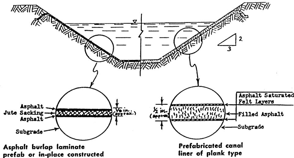
Figure 2. Type Section of an Exposed Membrane Lining (taken from Lauritzen, 1959, 1960).
