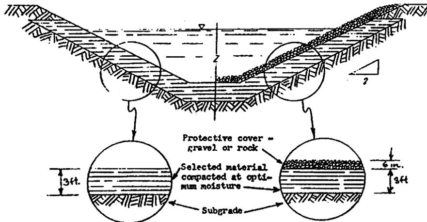
Figure 4. Type Section for Conditioned Earth Lining Method, with or without gravel cover (taken from Lauritzen, 1959, 1960)
