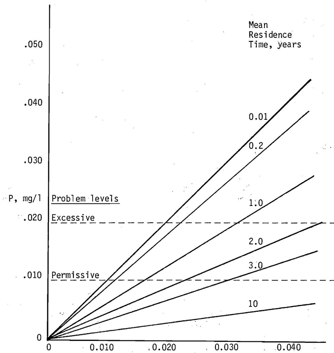
Figure 1. Relationship between phosphorus influent concentration (PI) and lake concentration (P) at different resident times (1/D, years). Net phosphorus removal (K) assumed to average 0.65. Calculated from mass balance form of steady state equation (Table 1). Problem levels based on Sawyer (1947).
