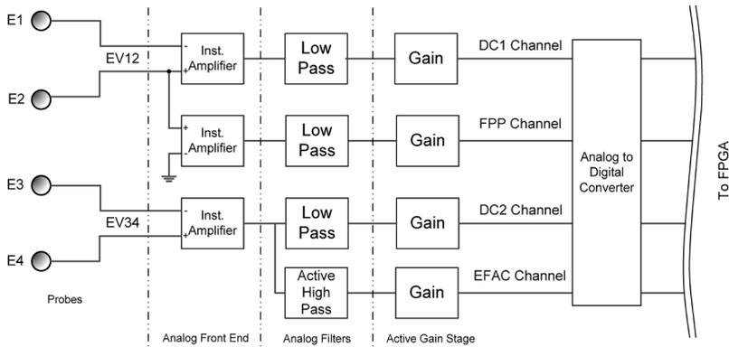
**Fig. 10** The DICE EFP functional block diagram
