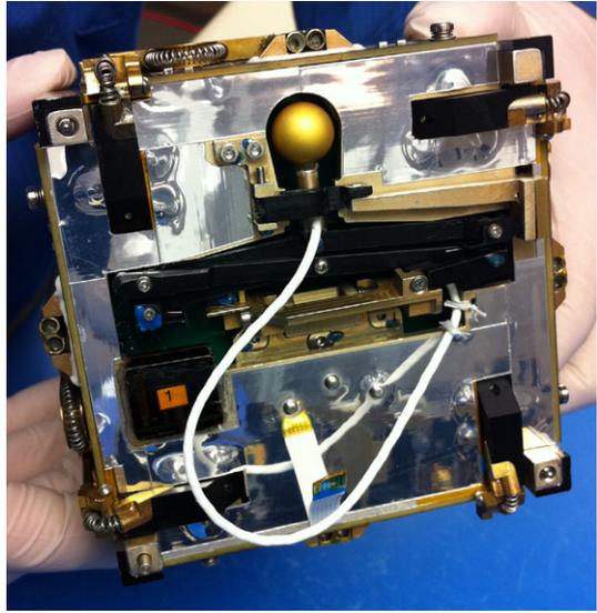
**Fig. 32** L-3 Comm's CadetU miniature radio is ideal for CubeSats and small satellites
