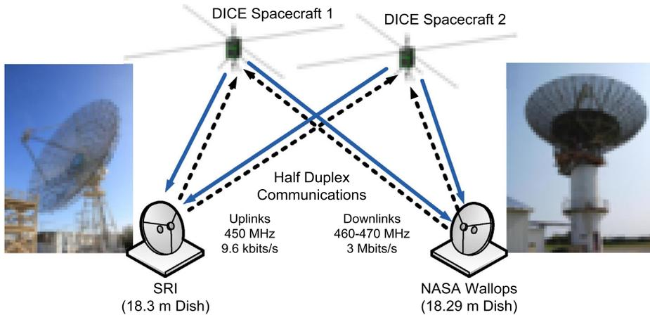
**Fig. 33** The DICE communications scenario uses the large UHF dishes at WFF and SRI to close the DICE high speed downlink
