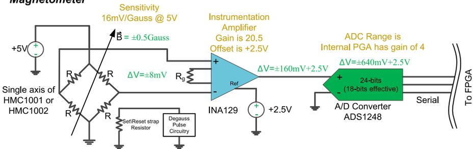
**Fig. 19** The DICE SciMag channel electronics schematic
