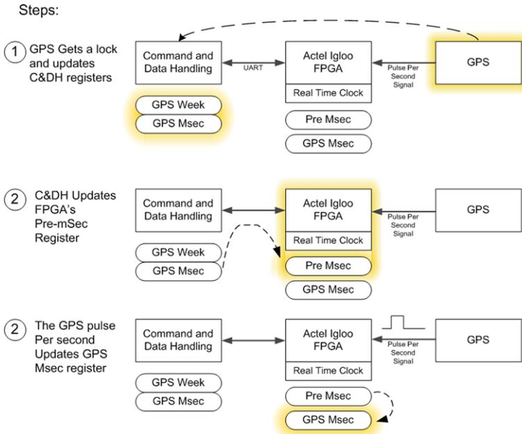
**Fig. 26** The DICE real time clock process was developed to maximize time stamp accuracy of the science measurements
