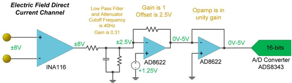
**Fig. 12** The DICE EFP DC channel electronics schematic
