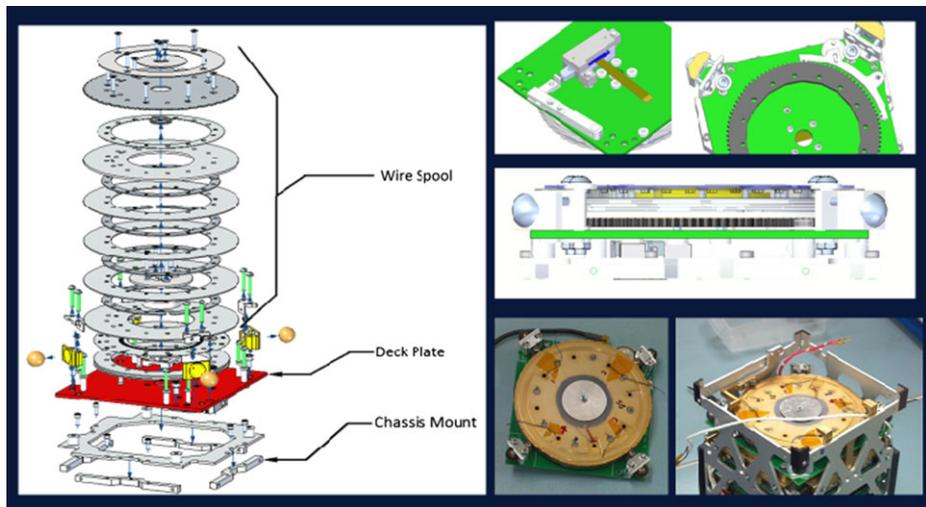
**Fig. 13** The DICE electric field boom deployment mechanism includes a set of precision spools, specialized cabling and harnessing, and non-magnetic motor actuator to deploy 5 m booms on orbit from spinning nano- and pico-satellite platforms
