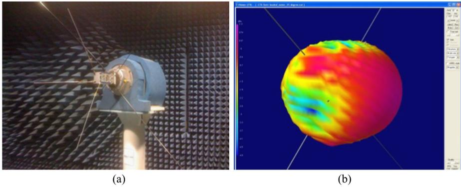
**Fig. 36** (a) The DICE antenna testing at NASA WFF; (b) The resultant antenna pattern is fairly uniform over all view angles (pattern is from a simulated model that closely matches the WFF test data), where the highest gain areas (pink) are 1.1 dBi and the lowest gain areas (dark blue) are  $-4.8$  dBi
