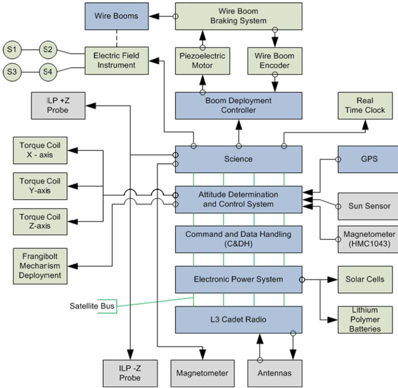
**Fig. 23** The DICE sensor-sat is a tightly coupled set of sub-systems that are controlled and managed via the C&DH
