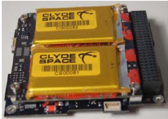
condition on the spacecraft and has the ability to recycle or switch off power to the remainder of the spacecraft upon detection of warnings, errors, or anomalies. The EPS maintains a nominal 8.2 V battery bus, and provides conditioned 5 and 3.3 V lines from the battery bus.
