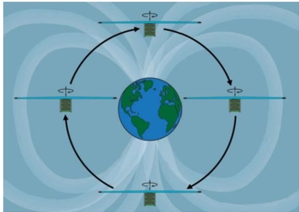
removal of the  $\mathbf{V} \times \mathbf{B}$  induced electric field component that is superimposed upon the target environmental electric field due to spacecraft movement through the geomagnetic field. The worst case  $\mathbf{V} \times \mathbf{B}$  induced electric field component is expected to be on the order of 350 mV/m, while the quiet time environmental EFP measurement capability is expected to be on the order of 0.5 mV/m. Each DICE spacecraft were designed to spin with the space-
