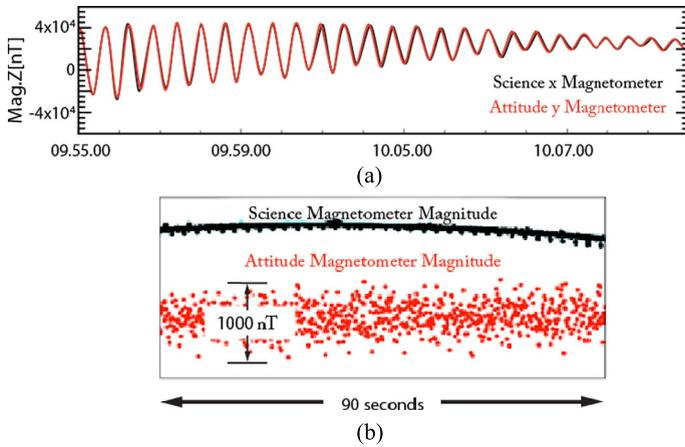
**Fig. 49** (a) Comparison of the DICE ADCS magnetometer and SciMag measurements on June 3, 2012; see Fig. 4 for the axes alignments of the two magnetometers; (b) a close up of the measurements, demonstrating the much lower noise ( $\sim 5\text{--}10$  nT) associated with the SciMag measurements
