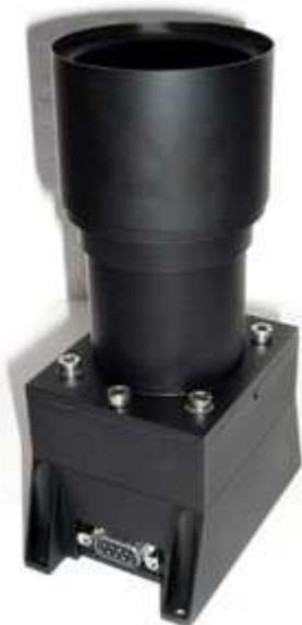
**Figure 3: ST-100 Star Sensor for LAPAN-A2 and LAPAN-ORARI**
