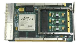
Figure 1 : Honeywell Responsive Digital Electronics (RDE) FPGA board
