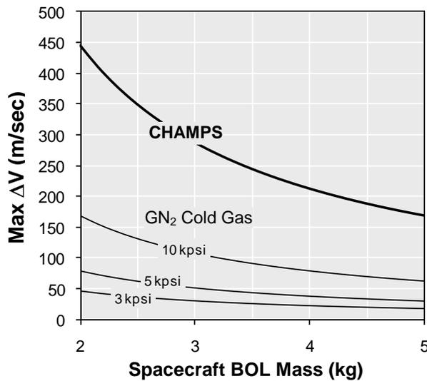
**Figure 7: Comparison of maximum deliverable  $\Delta V$  for CHAMPS and 3, 5, and 10 kpsi 1U GN<sub>2</sub> cold gas systems**
