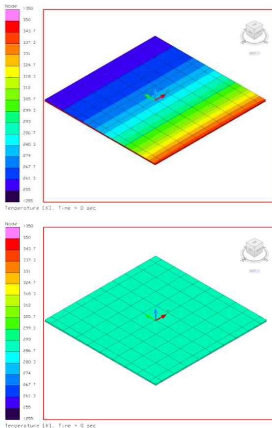
**Figure 13: Comparison of Aluminum Honeycomb (top) and TMT-Thermal Control Panel (bottom) 100 W Radiators (56 cm x 56 cm)**
