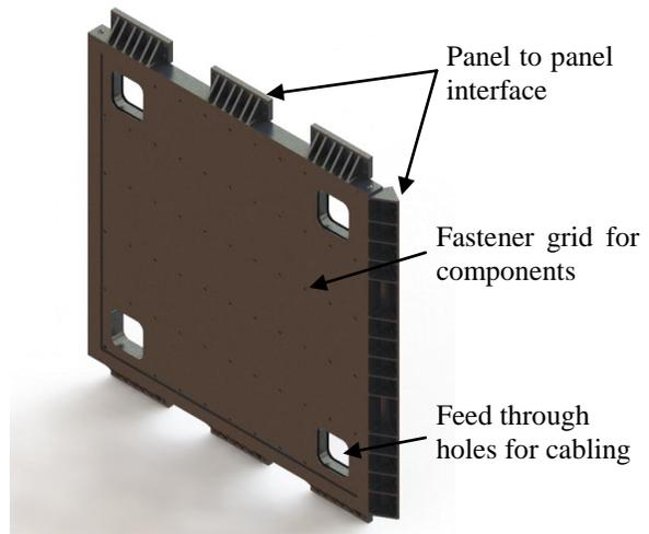
**Figure 11: Typical TCP for Structural-Thermal Applications**
