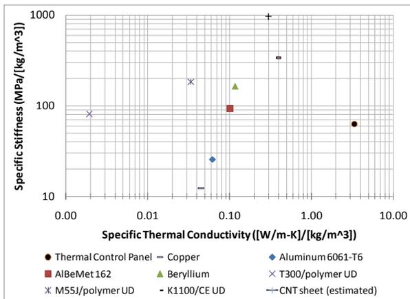
**Figure 10: Spacecraft Material Comparison (typical values)**
