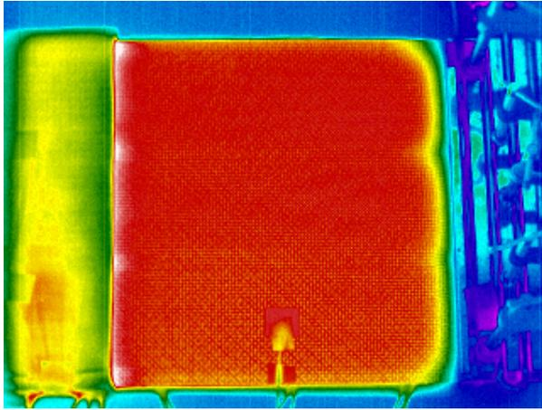
**Figure 9: IR View of Subscale Isothermal Skin Transferring 60 W from Left to Right**
