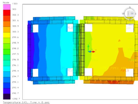
**Figure 5: Two panel; Panel heat load 56 W; Total Panel Delta T=3.8 C, Joint Delta T=2.5 C**
