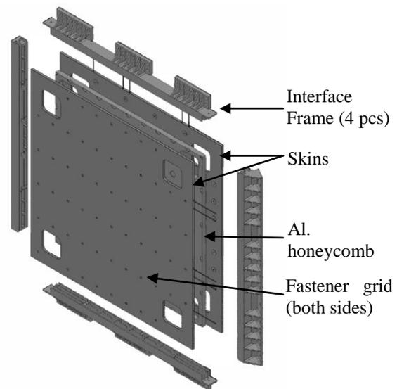
**Figure 3: Exploded View of Panel Configuration**
