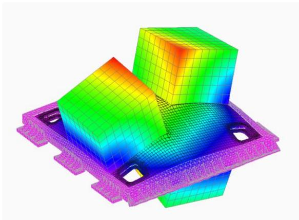
**Figure 7: First Mode Shape of TCP with Attached Masses**
