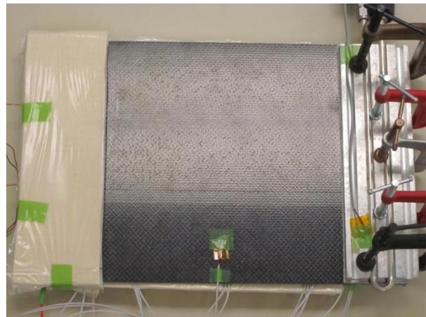
**Figure 8: Subscale Isothermal Skin Thermal Test Setup**
