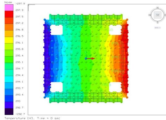
**Figure 4: Panel Temperatures; 56 W Input; Total Panel Delta T=4.5 C**
