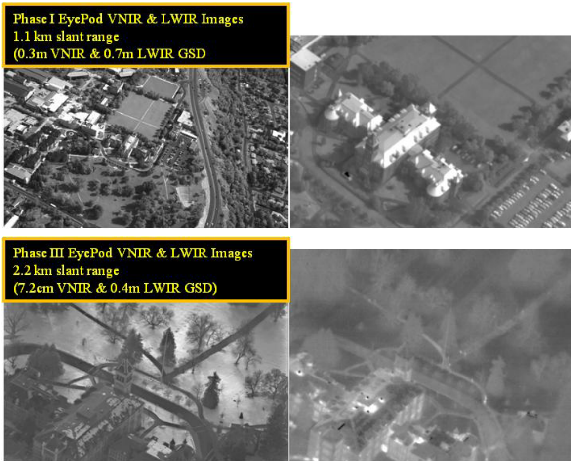
Figure 15. EyePod Phase I and Phase III VNIR and LWIR image of USU Old Main
