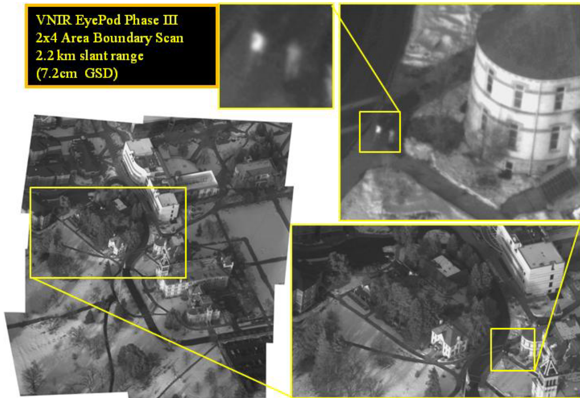
Figure 14. EyePod Phase III VNIR 2x4 area boundary collection over Old Main building on the campus of Utah State University, Logan, Utah (280 m x 250 m region)
