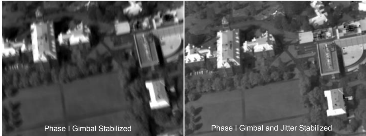
Figure 10. EyePod jitter stabilization mechanism turned off (left) and turned on (right).
