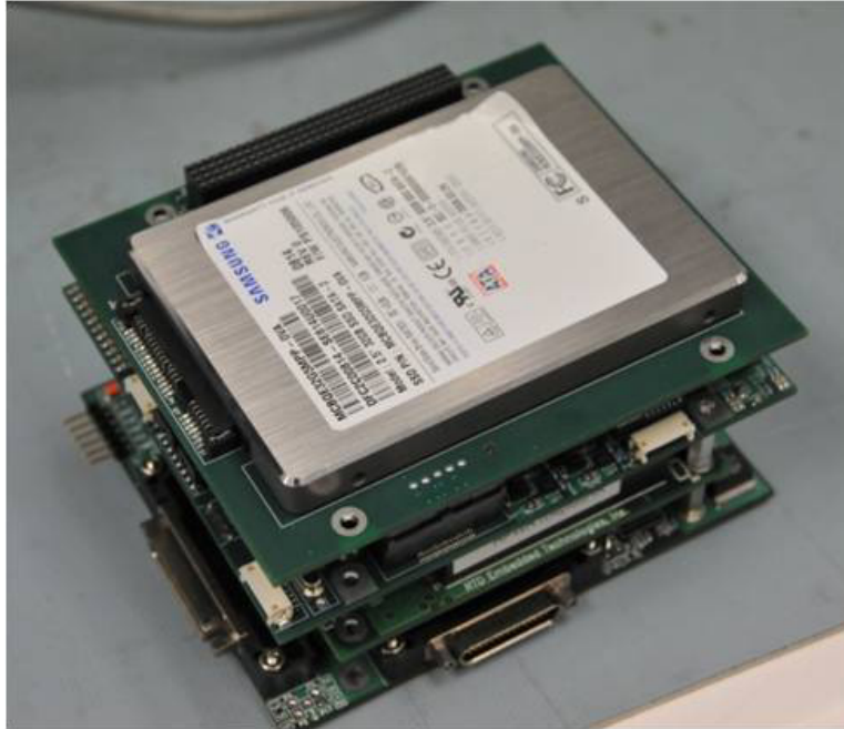
Figure 12. Processing stack including main stack, control stack, and SSD (4.55" x 3.775"x2")
