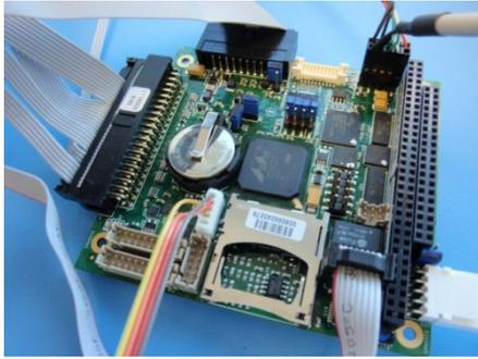
**Figure 8: Flight Computer**
