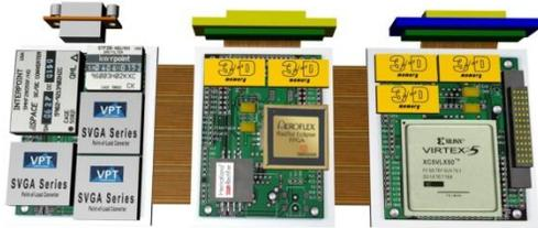
Figure 2 - SpaceCube MINI folded flat
