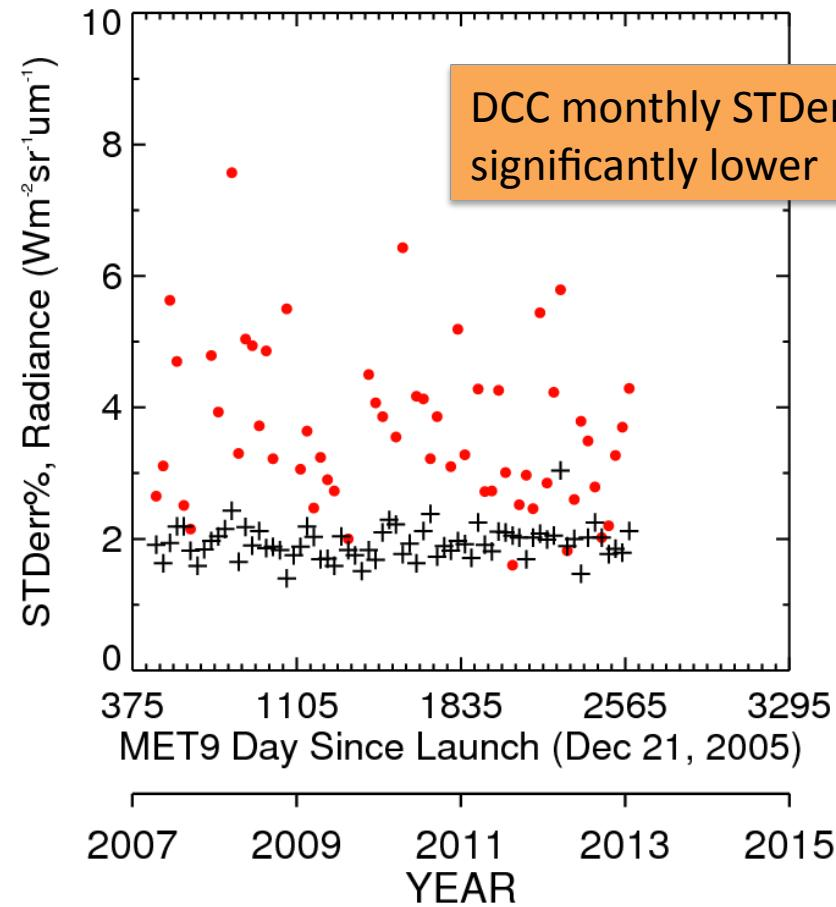
DCC ray-matching has the advantage of having a smaller SBAF, and a greater angle matching tolerance, which reduces the monthly stderr.
