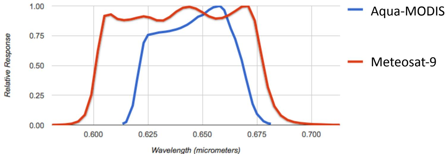
Must account for spectral response differences when inter-calibrating MODIS and Meteosat-9
