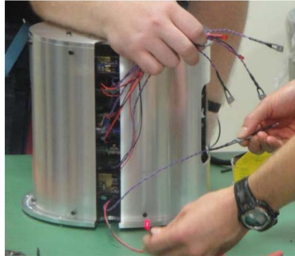
**Figure 6: RockSat Canister with 5 integrated RockOn Payload Plates (wire way visible)**
