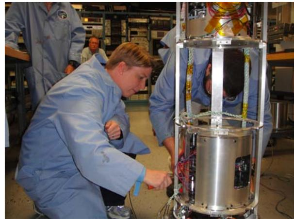
**Figure 7: RockSat Canister being integrated with rings and longerons**
