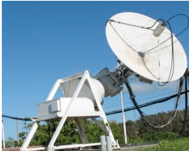
Figure 3.4: Palehua's 8-ft parabolic dish. This dish is used to monitor 1415, 2695, 4995, and 8800 MHz emissions from the sun.
