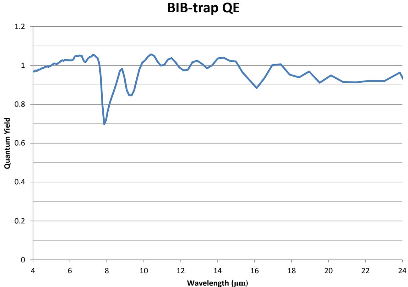
Spectral dependence of the quantum efficiency of a BIB-trap detector from calibration against the pyroelectric reference detector.
