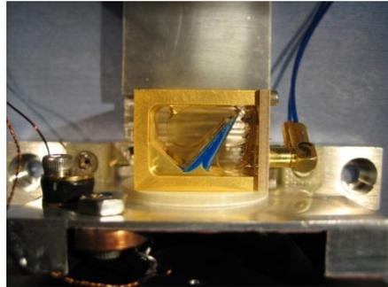
Trapping detector composed of two BIB (blocked impurity band) detectors, which exhibit significant responsivity from 2  $\mu\text{m}$  to 28  $\mu\text{m}$ .
