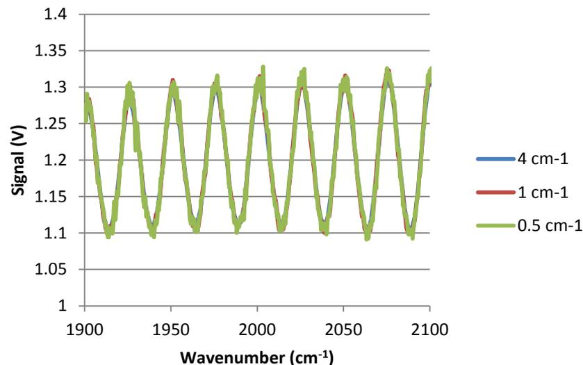
Spectral dependence of the response of a BIB detector taken with resolution of 0.5 cm<sup>-1</sup>, 1 cm<sup>-1</sup> and 2 cm<sup>-1</sup>. Shows etalon associated with interference effects from parallel planes of the detector.
