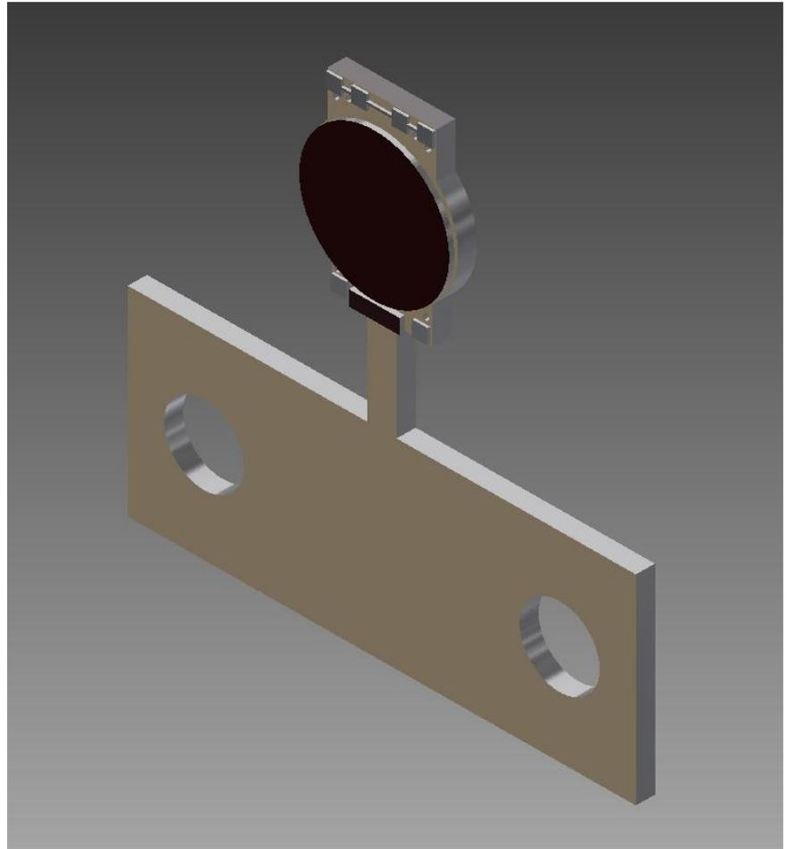
Planar ACR with Vertically-Aligned Carbon NanoTubes (VACNT) for the absorber. The VACNT material has reflectivity less than 0.2 % out to 18  $\mu\text{m}$ , and less than 1 % out to 50  $\mu\text{m}$ .
