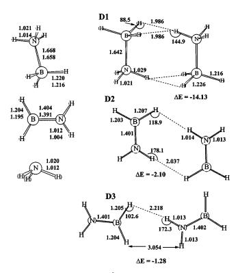
FIG. 1. Geometric parameters (in Å and degrees) of monomers and dimers of  $H_3BNH_3$  (**D1**) and  $H_2BNH_2$  (**D2** and **D3**), along with interaction energies ( $\Delta E$  in kcal/mol). The second set of values corresponds to the experimental geometries.
