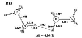
FIG. 9. Geometric parameters (in Å and degrees) of single dihydrogen bonded dimer of  $H_3BNH_3$ , along with interaction energies ( $\Delta E$  in kcal/mol).
