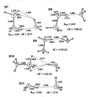
FIG. 3. Geometric parameters (in Å and degrees) and interaction energies ( $\Delta E$  in kcal/mol) of different isomers of  $H_3BNH_3-NH_3$  complexes. Numbers of negative frequencies are given in parentheses.
