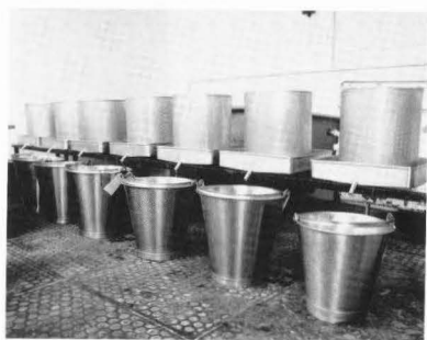
Fig. 2. An illustration of stainless steel perforated baskets and trays for the production of traditional Labneh.
