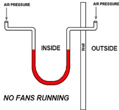
**Figure 1a.** No exhaust fans running (equal air pressure on inside and outside of building).
