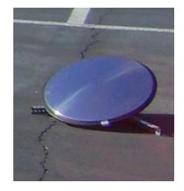
Schiller et al (2010, 2012) have used simple, convex, safety and truck side-view mirrors for calibration and characterization of satellite sensors
