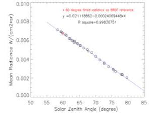
Figure 8. Dome C DNB BRDF linear fit.
