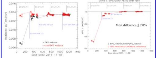
Figure 9. Dome C DNB radiance and reflectance of IDPS and Land PEATE data at 32x32 pixels area.
