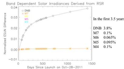
Figure 4. Normalized DNB and M bands ESUN values derived from modulated RSRs.
