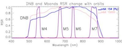
Figure 1. DNB and M bands prelaunch RSRs and modulated RSRs.
