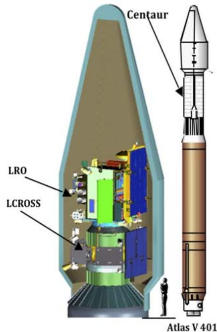
**Figure 2: The LRO/LCROSS Launch Vehicle Stack**
