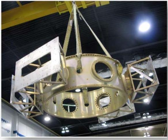
**Figure 7: LCROSS ESPA Ring and Secondary Panels**
