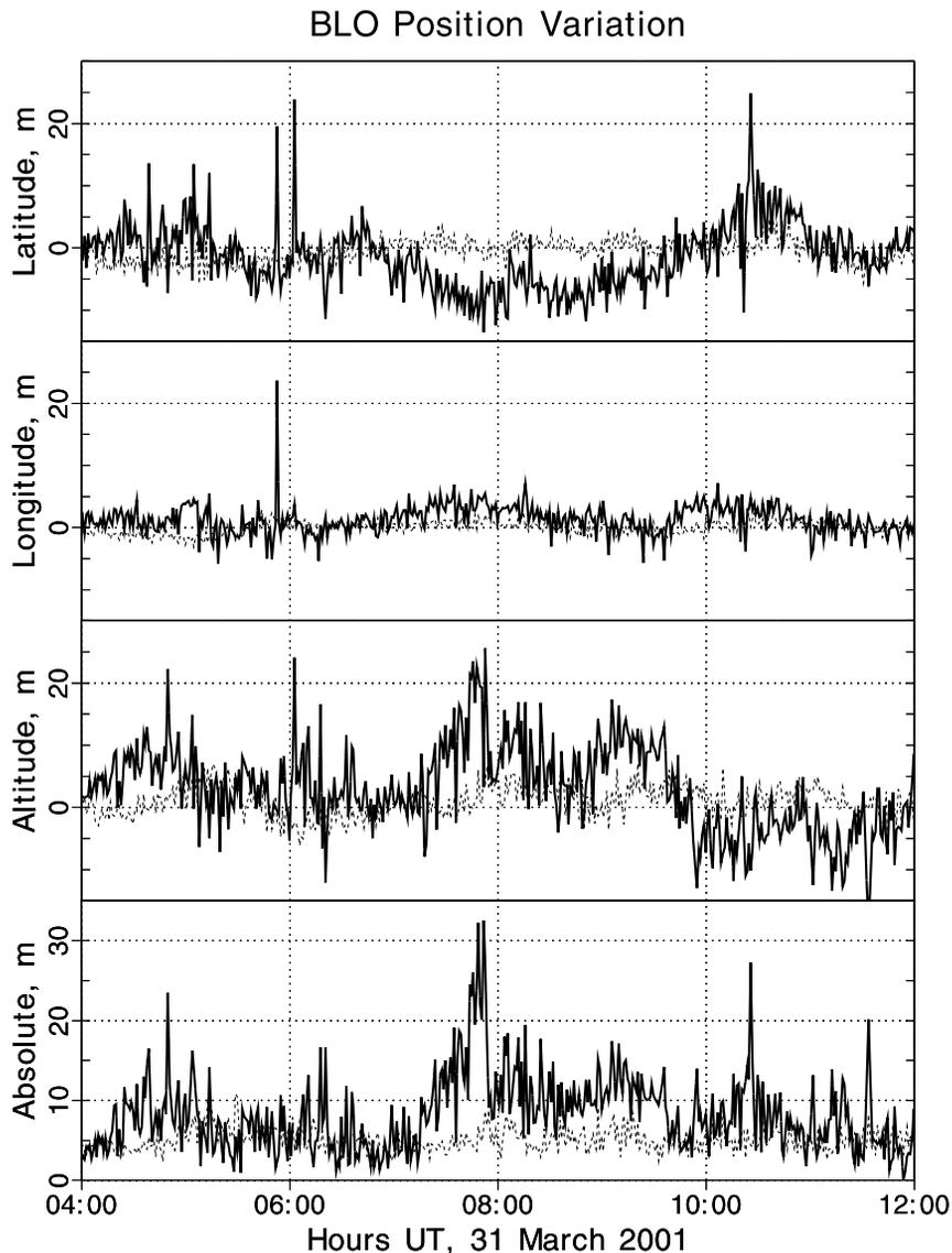
Figure 6. BLO GPS single-frequency geolocation coordinate errors and (bottom) absolute error from 0400 to 1200 UT on 31 March 2001 (solid line) compared with the median value of the previous 6 days (dashed line).
