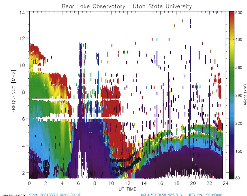
**Figure 4.** BLO dynasonde observations of the ionosphere from 0000 to 2400 UT on 31 March 2001. The individual ionograms are vertical color-coded lines in which color represents virtual height (km) and the vertical axis is the sounding frequency (MHz).
