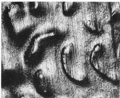
Figure 19. Using DIC optics, flange (19A) and lid (19B) seal activation patterns were visible on a cup sealed with a coextruded film type sealant.
